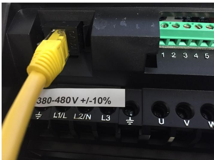
*The connecting cable plugs into the MPC's expansion socket which is located to the left of the green control terminal strip inside the terminal cover of the MPC.*
